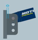
Double check clearance between ram and mounting plates
