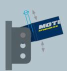
Check clearance between ram base and flanges on mounting plates
